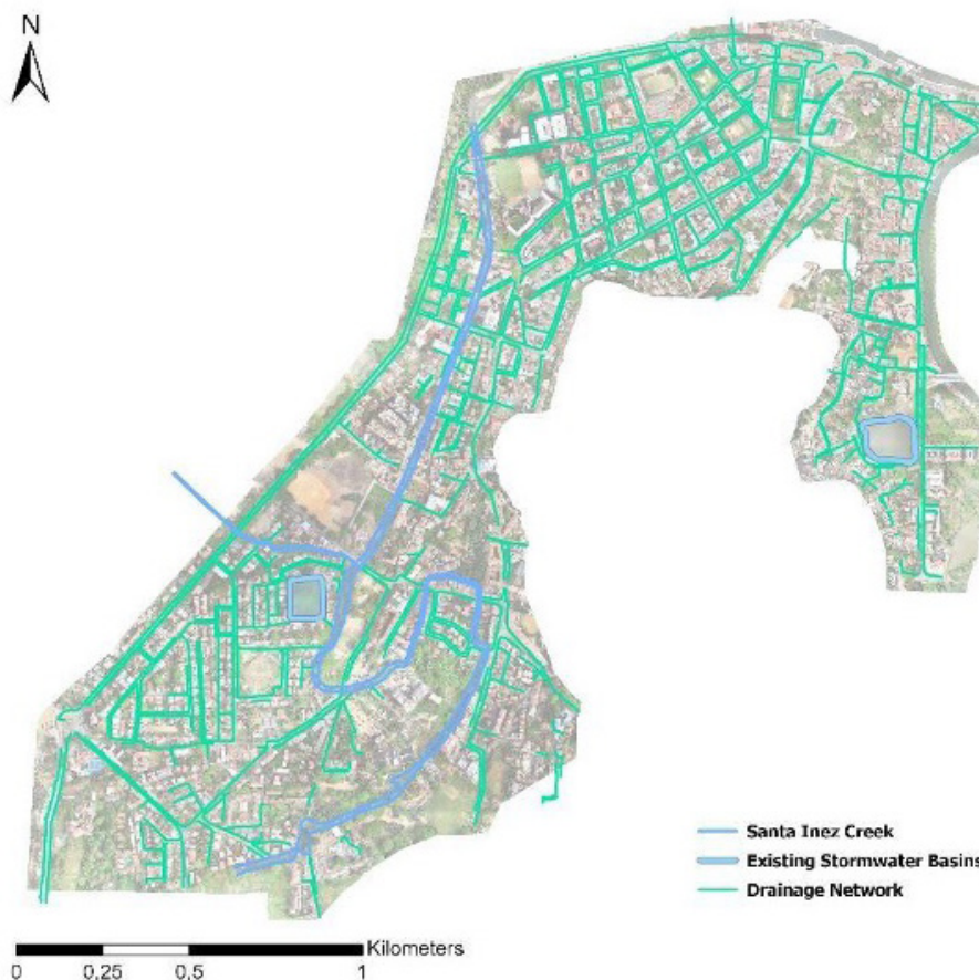
Figure 01: Modelling approach that includes the drainage system, relying on simplifications and assumption to simulate the hydrology and hydraulics of surface flows.
