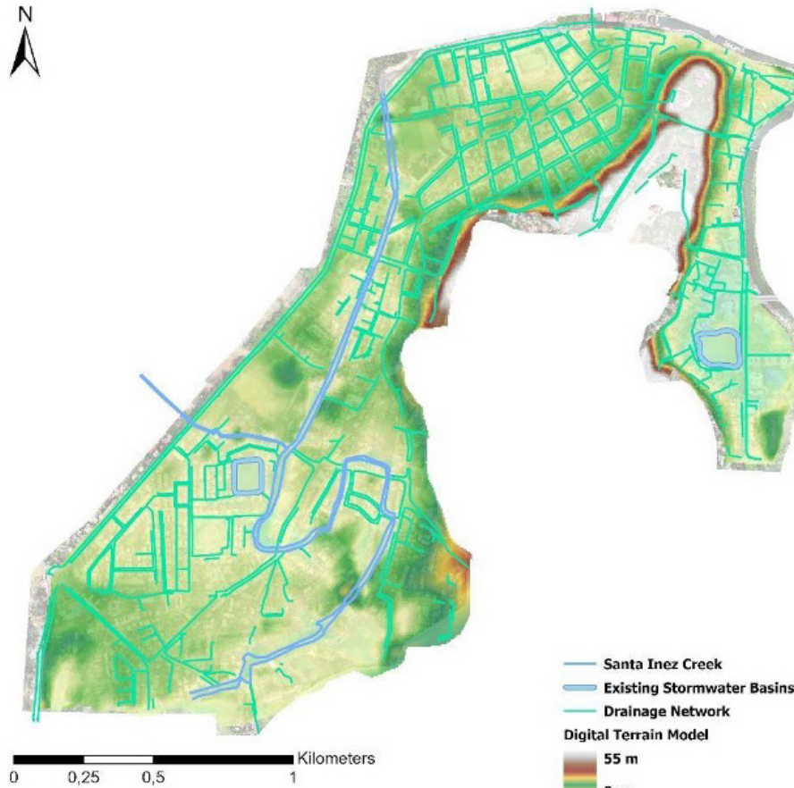
Figure 01: Modelling approach that includes the drainage system and terrain relying on simplifications and assumptions to simulate hydrological conditions such as infiltration and evaporation
